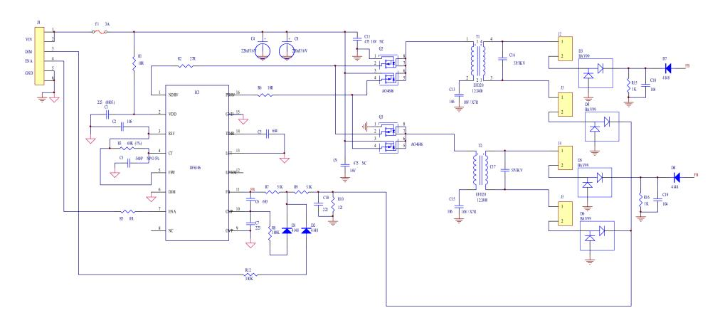
VIN: 108—13.2 V ENA: 0-1V OFF, 2-5V ON; DIM: 0-5V Analog Mode, 0V MAX, 5V MIN Lamp Voltage 650 Vrms Lamp Curent 6.5 mArms Operation frequency 52.0 KHz Test Panet: 19 Hanster HSD 190ME13
