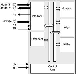
**Exponent** – performs operations on exponent part of number. The addition, subtraction, shifting, comparison and conversion operations are executed in this module. It contains exponents and work registers.
