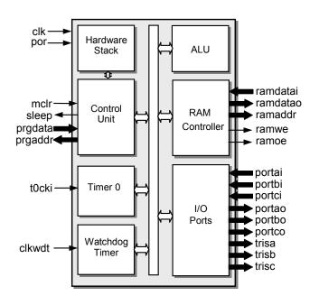
**ALU** – Arithmetic Logic Unit performs arithmetic and logic operations during execution of an instruction. This module contains work register (W) and Status register.
