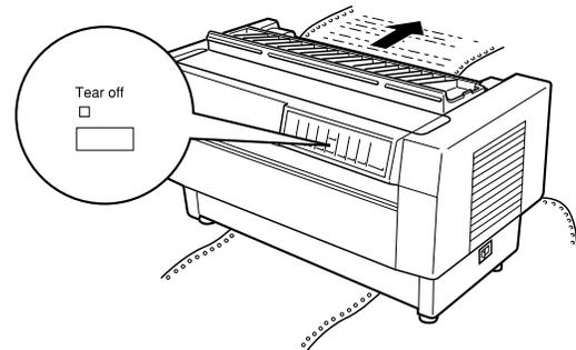
4. If the paper is not aligned with the tear-off edge, press the **Micro Feed** buttons to feed the paper forward or backward in 1/216-inch increments. (You can also hold down either **Micro Feed** button to feed the paper continuously.)
