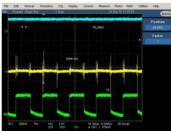
Figure 32. During startup, current is high, with shorted COM-VSS, noise is less, fault conditions do not occur, compressor will not stall, 100µs/div
