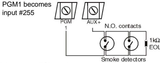
When using ESL smoke detectors with the CleanME™ feature, do not connect more than 20 detectors in parallel.
