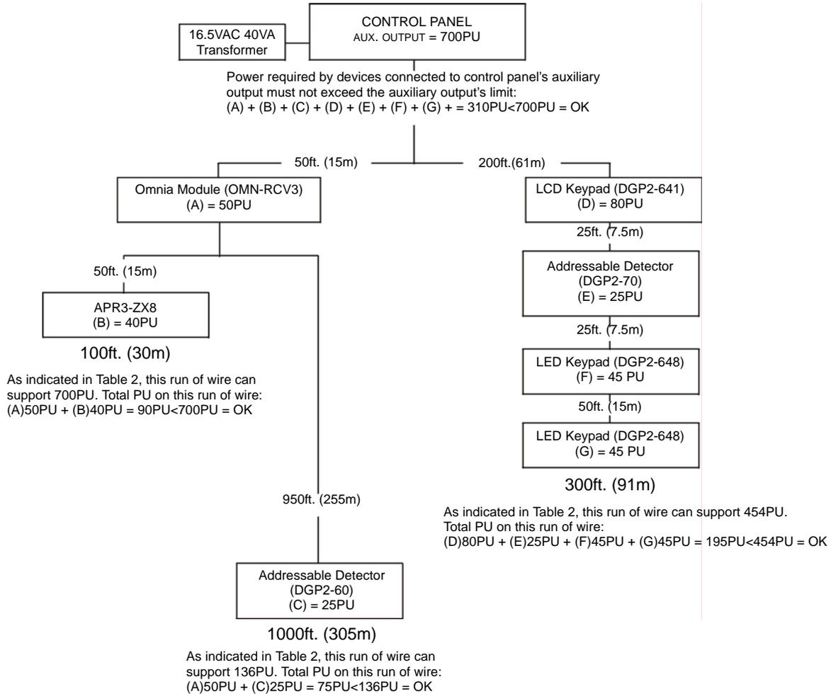
If in the above example you were to add an LCD Keypad (80PU) to the 100 foot or 300 foot wire, you would not exceed the wire's limit. Although, adding the LCD Keypad to the 1,000 foot wire would exceed the wire's limits, thereby causing devices to function at decreased capacity.
