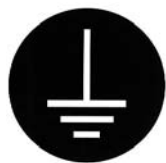
Compulsion, connect to the grounding terminal
