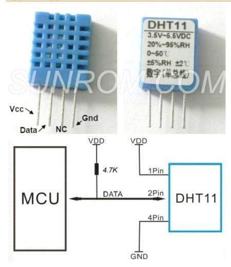
DHT11's power supply is 3-5.5V DC. When power is supplied to the sensor, do not send any instruction to the sensor in within one second in order to pass the unstable status. One capacitor valued 100nF can be added between VDD and GND for power filtering.
