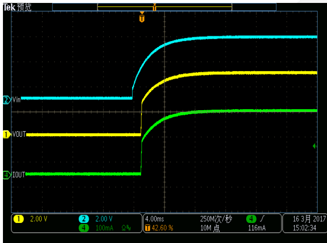
No-Load to Over-Load Transient Response ( V_{in}=5\text{V} , R_{load}=2.7\text{ohm} )
