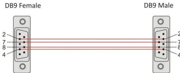
Figure 27 – Building an extension cable
