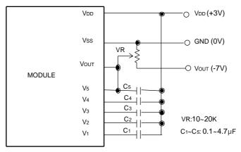
Both the boosting circuit and the voltage control circuit are not used in this module. Therefore, connect V<sub>5</sub> pin with Vout pin and supply the LCD driving voltage from the outside.
