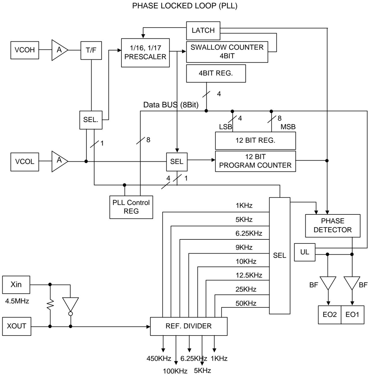
Figure 5-7 PLL Block Diagram
