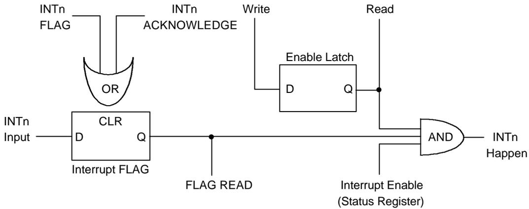
Figure 5-4A-1. Interrupt Logic
