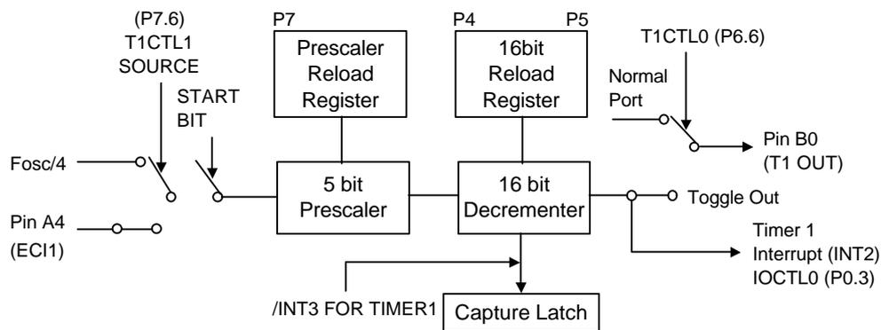
Figure 5-5. Timer 1 Schematic Diagram
