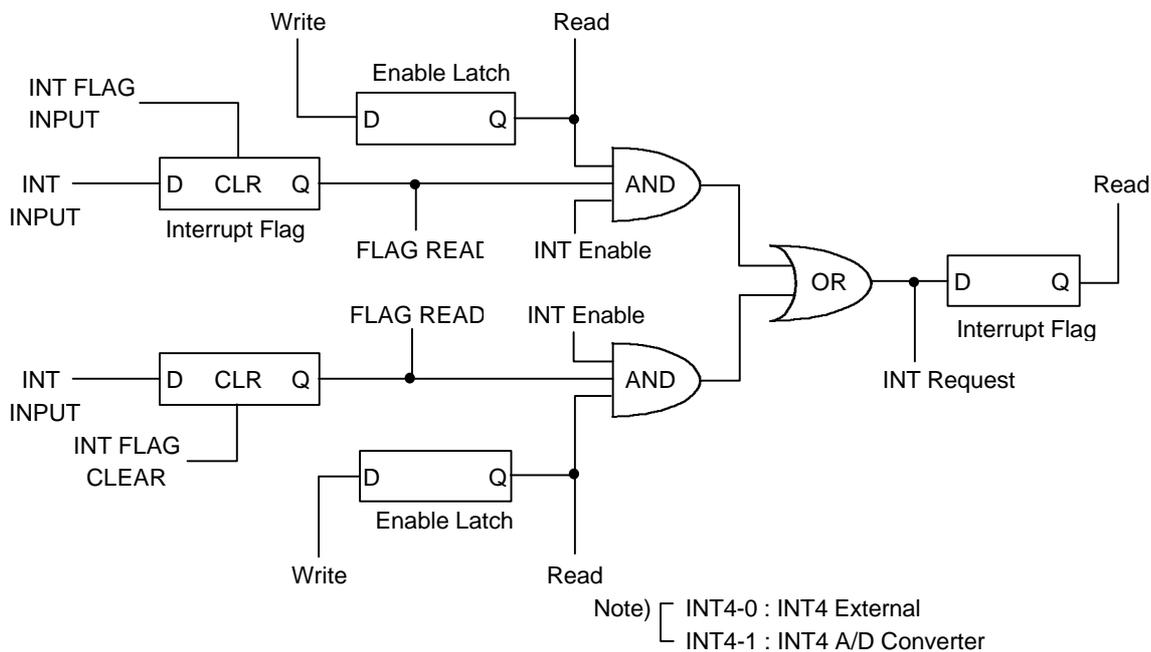
Figure 5-4A-2. Interrupt 4 Logic
