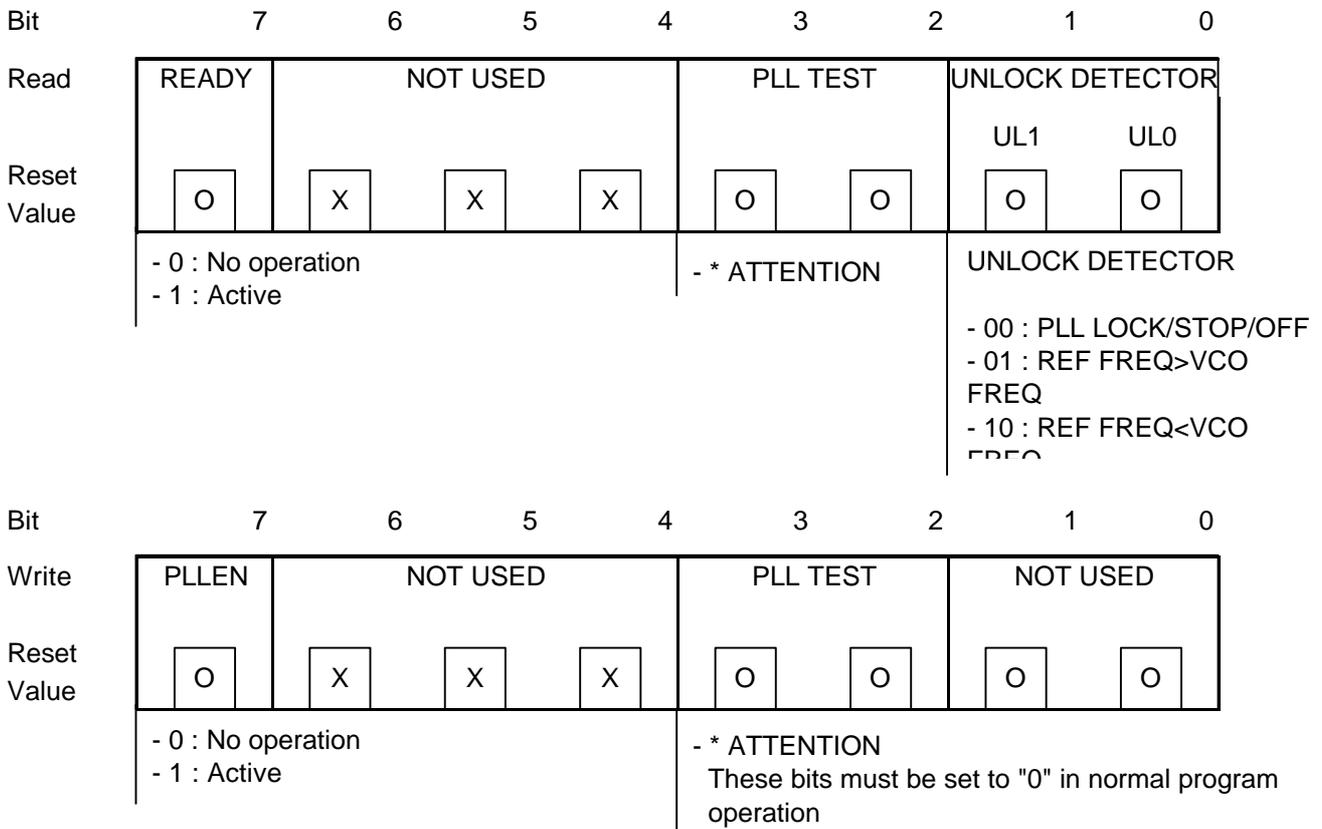
Figure 5-7-5. PLL Control Register
