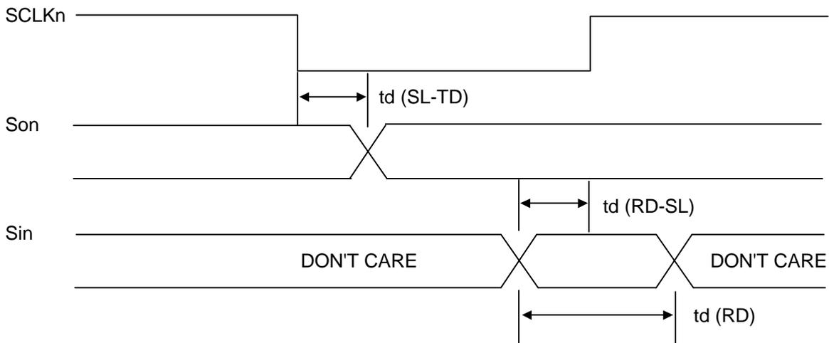
Figure 7.2 AC Characteristics for Serial I/O ports
