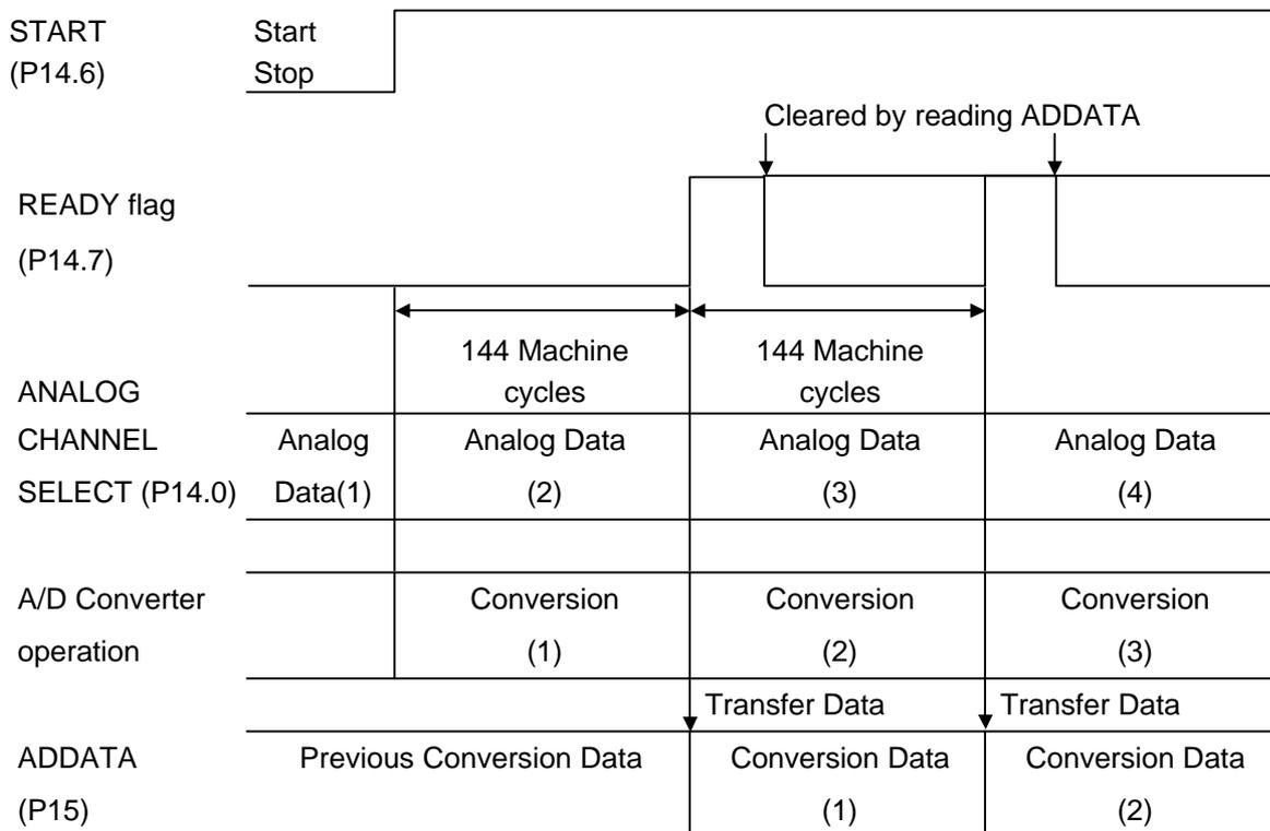
Figure 5-9 Continuous A/D Conversion
