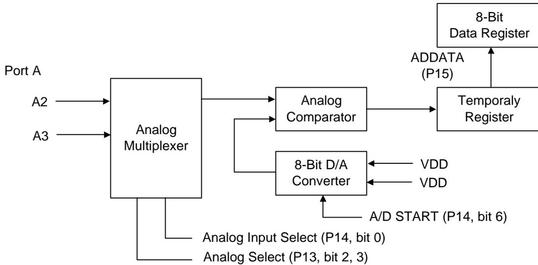
Figure 5-7. A/D Converter Function Block Diagram
