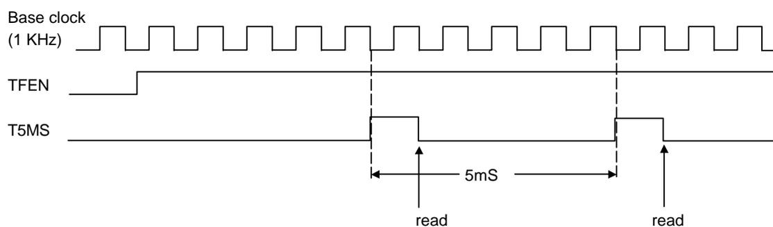
T250MS, T125MS, T100MS, T5MS : Interval timer flag bits.
