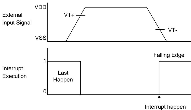
Figure 5-4B External Interrupt Timing
