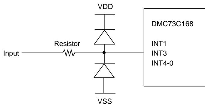
Figure 5-4C Additional Circuitry for External Input
