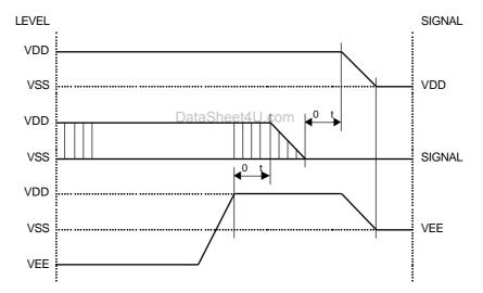
Please maintain the above sequence when turning on and off the power supply of the module. If VEE is supplied to the module while alternate signal for LCD driving (M) is unstable, DC component will be supplied to the LCD panel. This may cause damage the LCD module.
