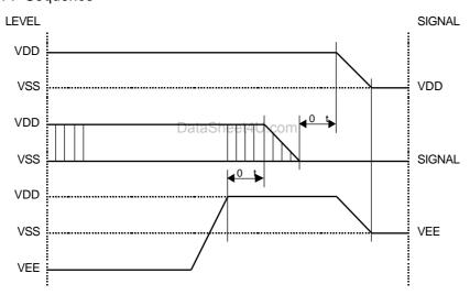
Please maintain the above sequence when turning on and off the power supply of the module. If VEE is supplied to the module while internal alternate signal for LCD driving (M) is unstable, DC component will be supplied to the LCD panel. This may cause damage the LCD module.
