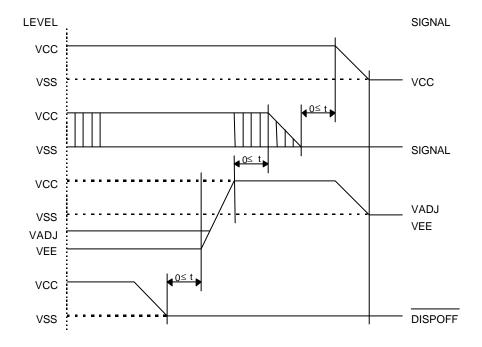
Please maintain the above sequence when turning on and off the power supply of the module.
