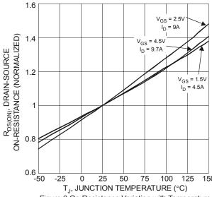
Figure 6 On-Resistance Variation with Temperature
