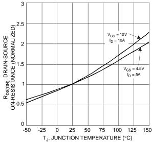
Figure 6 On-Resistance Variation with Temperature
