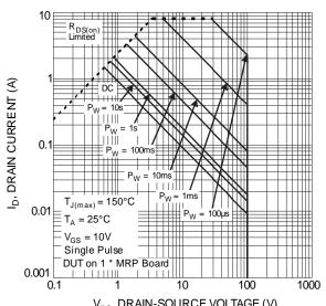
$\rm V_{DS}^{}$ , DRAIN-SOURCE VOLTAGE (V) Figure 12 SOA, Safe Operation Area
