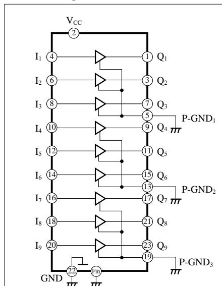
Note) GND, Fin, P-GND 1, 2, and 3 are connected inside the IC, but be sure to connect them outside for use.
