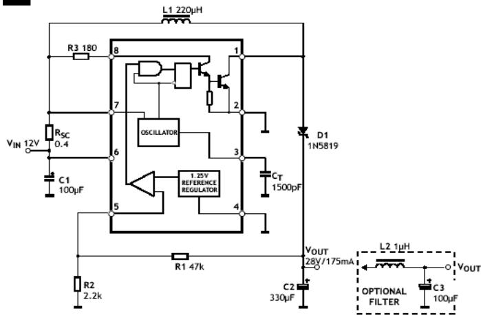
This is a typical step-up converter configuration. In the steady state, if the resistor divider voltage at pin 5 is greater than the voltage in the non-inverting input, which is 1.25V determined by the internal reference, the output of the comparator will go low. At the next switching period, the output switch will not conduct and the output voltage will eventually drop below its nominal voltage until the divider voltage at pin 5 is lower than 1.25V.
