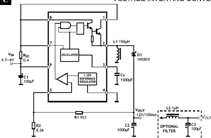
This is a typical inverting converter configuration. The working process in the steady state is similar to step-up converter, the difference in this situation is that the voltage at the non-inverting pin of the comparator is equal to  $1.25V + V_{OUT}$ , then  $V_{pin5} = V_{OUT} * R2/(R1+R2) = 1.25V + V_{OUT}$ , so the output voltage can be decided by  $V_{OUT} = -1.25 * (R1+R2)/R1 (V)$ .
