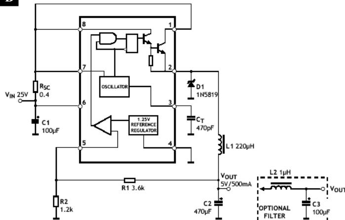
This is a typical step-down converter configuration. The working process in the steady state is similar to step-up converter,  $V_{pin5} = V_{OUT} * R2/(R1+R2) = 1.25 (V)$ , the output voltage can be decided by  $V_{OUT} = 1.25 * (R1+R2)/R2 (V)$ .
