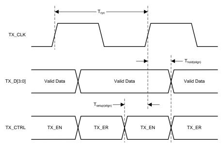
Figure 5. RGMII Transmit Timing (Internal Delay Disabled)
