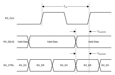
Figure 6. RGMII Receive Timing (Internal Delay Enabled)
