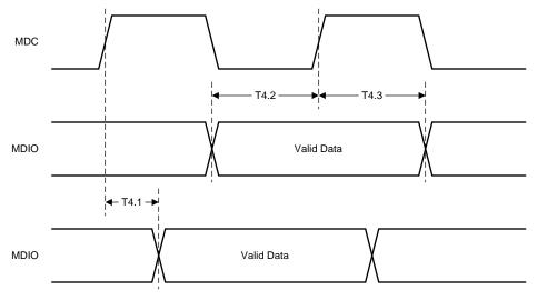
Figure 8. Serial Management Timing
