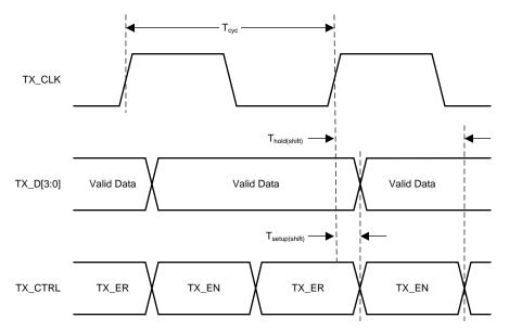
Figure 4. RGMII Transmit Timing (Internal Delay Enabled)
