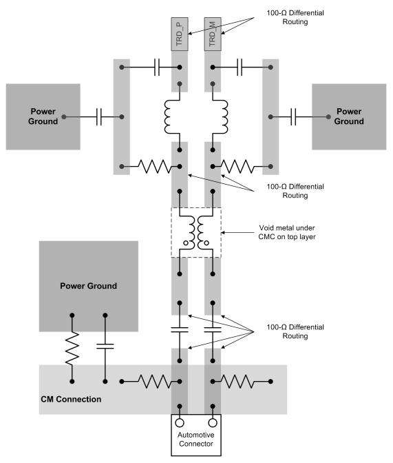
Figure 146. MDI Low-Pass Filter Layout Recommendation
