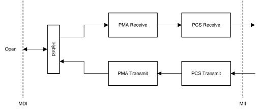
Figure 21. Analog Loopback
