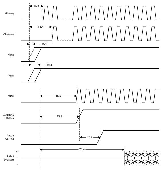
Figure 9. Power-Up Timing
