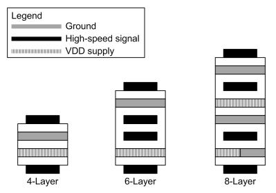
Figure 144. Recommended PCB Layer Stack-Up
