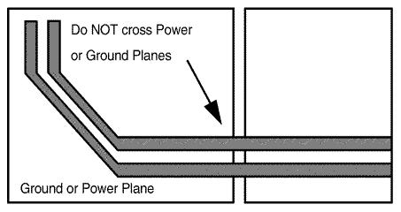
Figure 143. Power and Ground Plane Breaks
