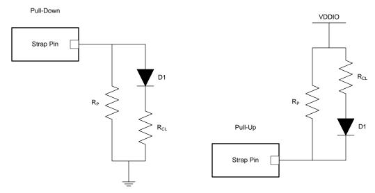
Figure 28. Example Strap Connections
