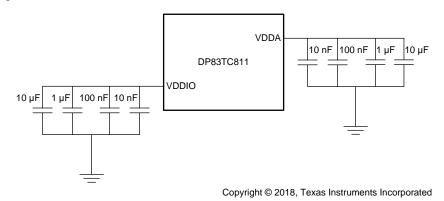
Figure 141. Recommended Supply De-Coupling Network
