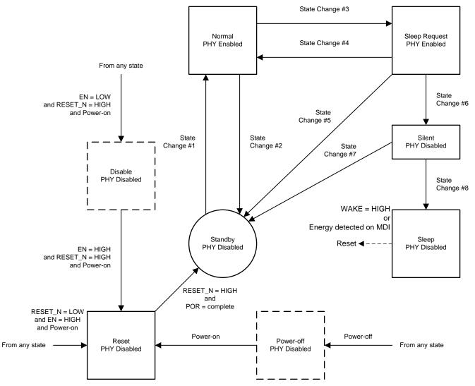
Figure 23. PHY Operation State Diagram
