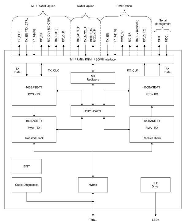
Figure 15. DP83TC811R-Q1 Functional Block Diagram
