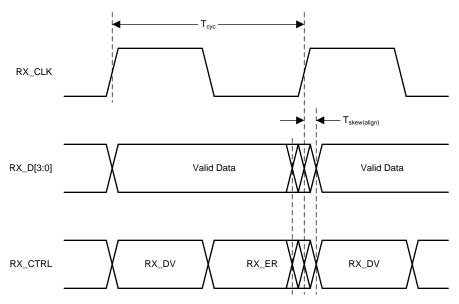
Figure 7. RGMII Receive Timing (Internal Delay Disabled)
