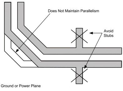
Figure 142. Differential Signal Trace Routing
