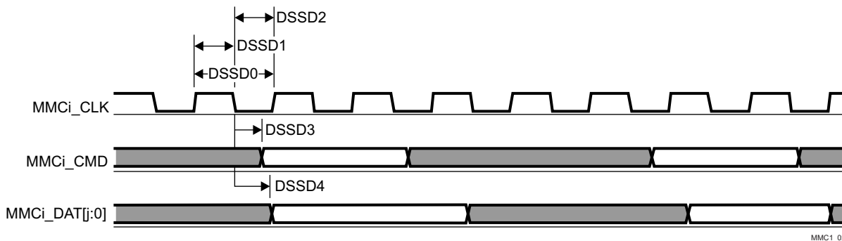
Figure 5-87. SD/SDIO in – Default Speed – Transmitter Mode
