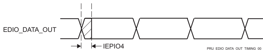
Figure 5-120. PRU_ICSSG IEP Digital IOs Timing
