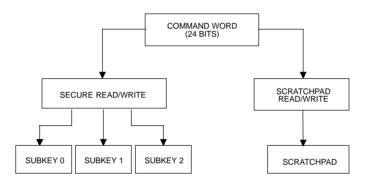
The 24 bit function command word is organized into three fields of eight bits each. These one byte fields include the function to be performed, the memory partition to be accessed and the starting byte address for the data transfer operation. The starting byte address and the partition codes are required to be given in both real and complement form. If these values do not match, access to the part will be denied (Figure 2).
