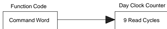
SEQUENCE: PROGRAM MODE, READING THE 9-BIT NUMBER OF DAYS COUNTER Figure 6B
