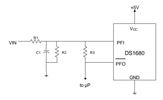
$$V_{TRIP} = 1.25 \left( \frac{R1 + R2}{R2} \right) \qquad V_{H} = 1.25 / \left( \frac{R2||R3}{R1 + R2||R3} \right)$$
