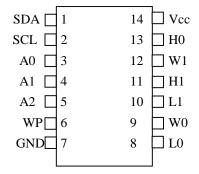
14-Pin TSSOP (173 mil) 14-Pin Flip Chip (100 x 100 mils) 16-BALL STPBGA (4 x 4 mm) See Mech. Drawing Section
