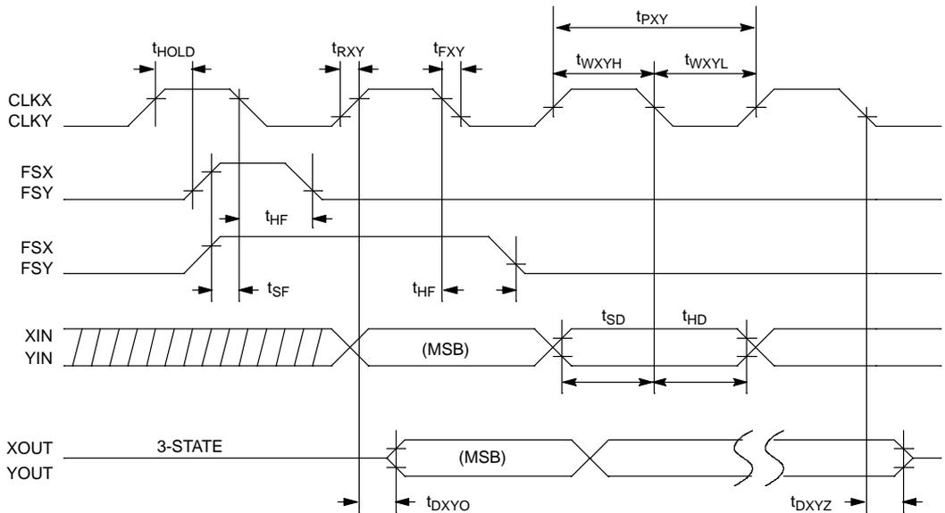
**MASTER CLOCK/RESET AC TIMING DIAGRAM** Figure 14
