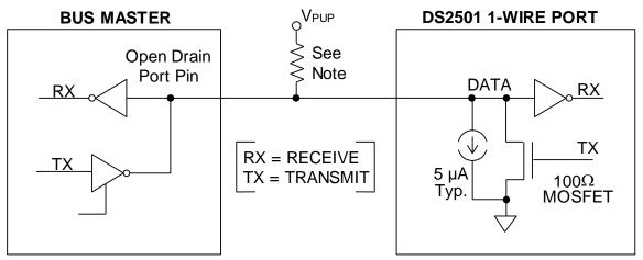
Note: Depending on 1-Wire communication speed, regular or overdrive, and bus load characteristics, the optimal pull-up resistor value will be in the  $1.5k\Omega$  to  $5k\Omega$  range.
