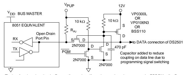
The interface is reduced to the Rpu pull-up resistor if one does not intend to program the EPROM cells. Rpu will be in the 1.5K to 5K range depending on bus load characteristics
