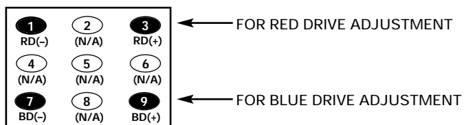
Figure 6. Remote Control Number keys' functions in Service Menu NO. 72 DRV
