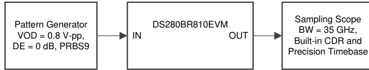
Figure 11. Minimal Rx/Tx Channel Test Setup
