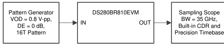
Figure 23. FIR Test Setup
