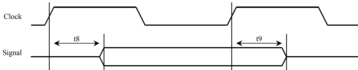
Figure 18-5. To/From Hi Z Delay Definitions (Rising Clock Edge)
