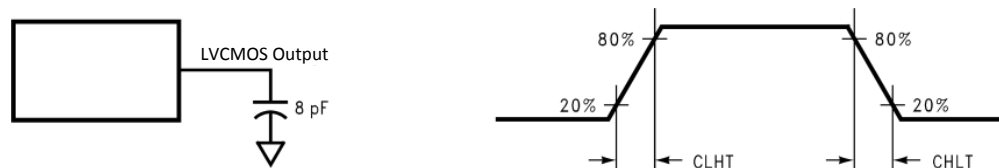
Figure 2. LVC MOS Output Load and Transition Times
