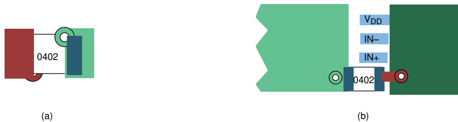
Figure 11-7. Typical Decoupling Capacitor Layouts
