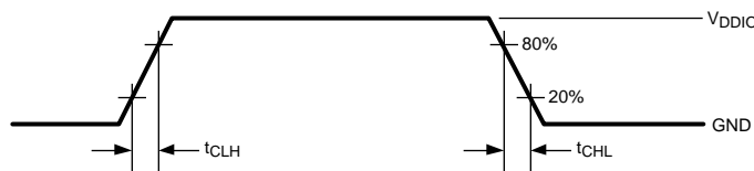
Figure 3. LVCMOS Transition Times
