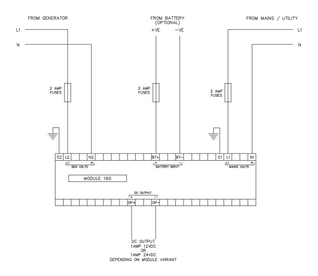
TERMINALS SUITABLE FOR 22-16 AWG  $(0.6 mm^2 - 1.5 mm^2)$  FIELD WIRING TIGHTENING TORQUE = 0.8 Nm (7lb-in)
