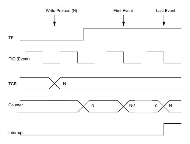
Figure 8-16 Mode 7 — Standard Timer Mode, External Clock (INV=1)
