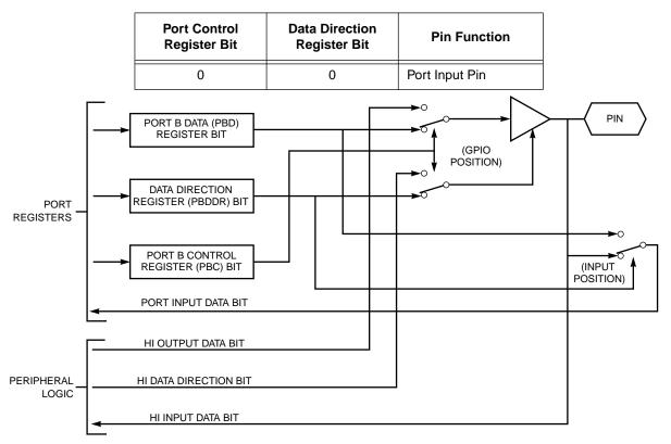
Figure 5-4 Port B I/O Pin Control Logic
