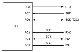
Figure 7-32 Continuous Clock — Asynchronous Operation
