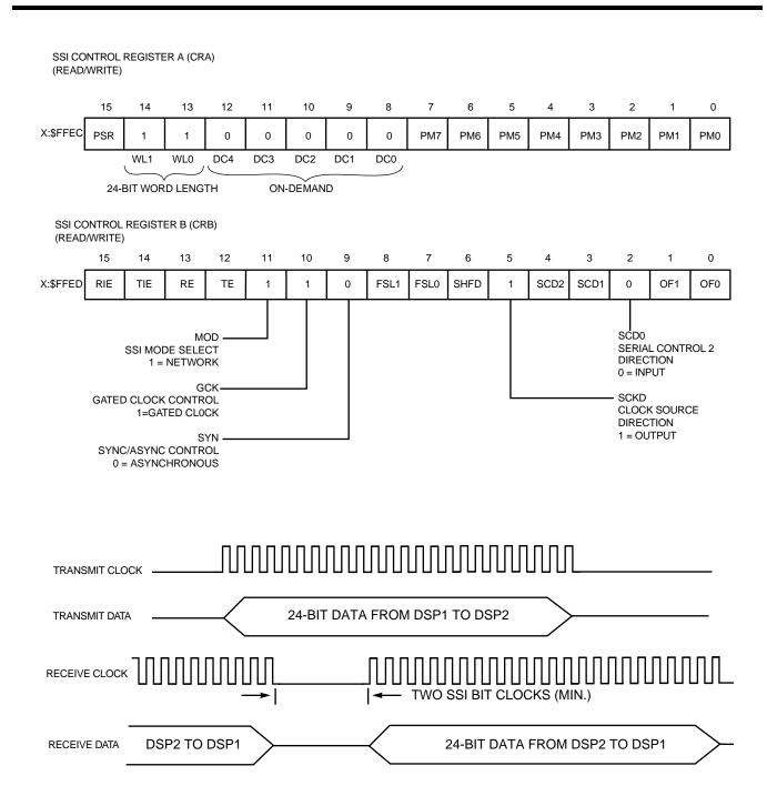
**NOTE:** Two SSI bit clock times are automatically inserted between each data word. This guarantees frame sync will be low between every data word transmitted and the clock will not be continuous for two consecutive data words.
