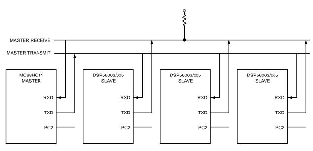
Figure 6-41 Master-Slave System Example
