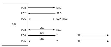
Figure 7-30 Gated Clock — Asynchronous Operation
