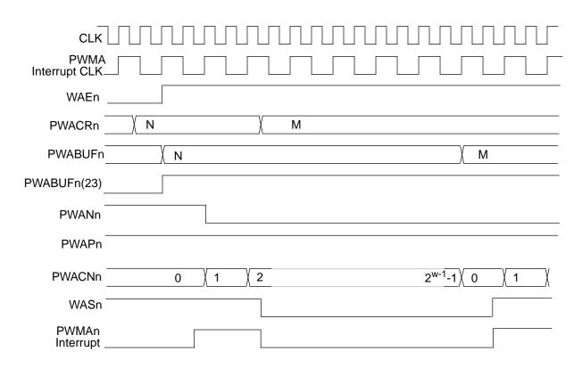
Figure 9-12 PWMA Timing — Internal Clock, Internal Carrier, N=\$8000, w=16
