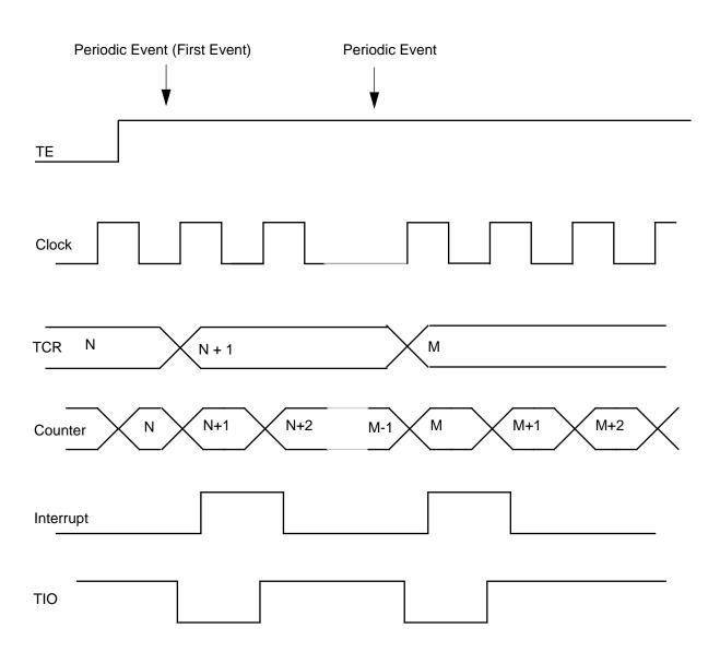
Figure 8-12 Mode 5 — Period Measurement Mode (INV=1)
