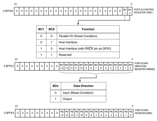
Figure 5-2 Parallel Port B Registers
