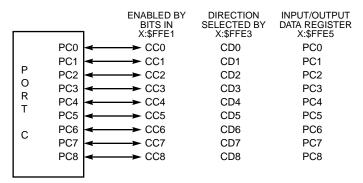
Figure 7-2 Port C GPIO Control
