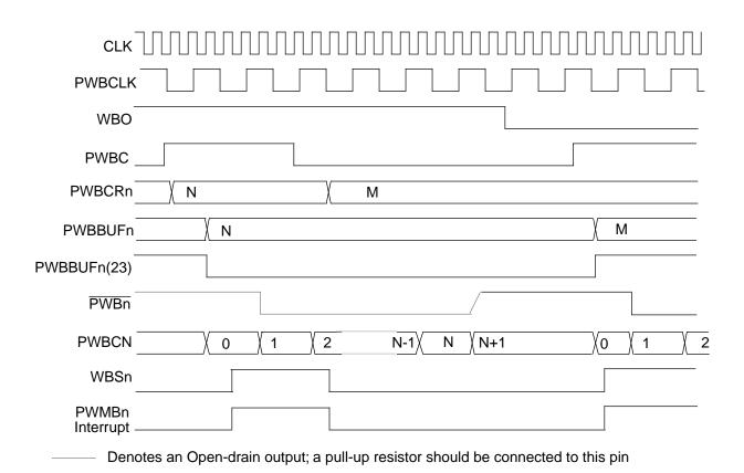
Figure 9-14 PWMB Timing — External Clock, External Carrier
