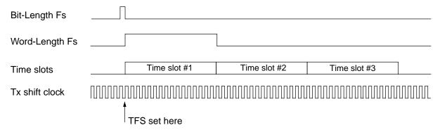
Data written to the transmit data register during the time slot when TFS is set will be transmitted (in network mode) during the second time slot in the frame. TFS is useful in network mode to identify the start of the frame. This is illustrated in a typical transmit interrupt handler:
