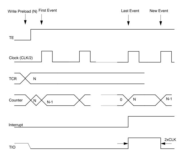
Figure 8-5 Mode 1 — Standard Timer Mode, Internal Clock, Output Pulse Enabled (INV=0)
