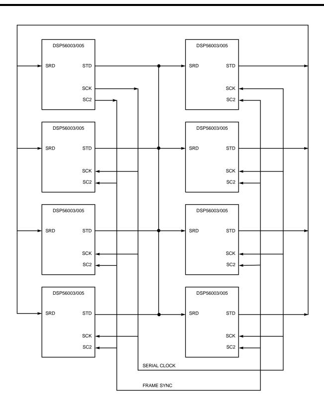
**Figure 7-59** SSI TDM Connected Parallel Processing Array direction that data is transferred in the matrix (north, south, east, or west).
