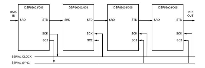
Figure 7-57 SSI Cascaded Multi-DSP System
