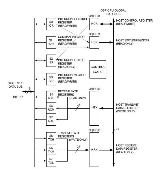
Figure 5-8 HI Block Diagram
