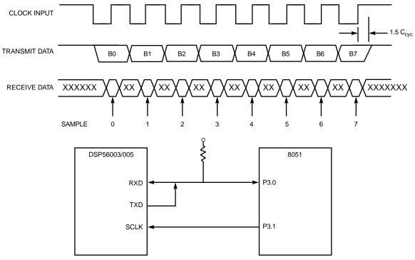
Figure 6-39 Synchronous Mode Example
