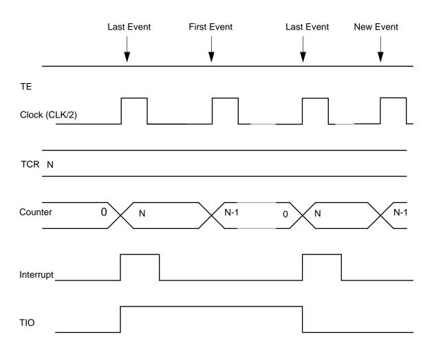
**Figure 8-7** Mode 2 — Standard Timer Mode, Internal Clock, Output Toggle Enable
