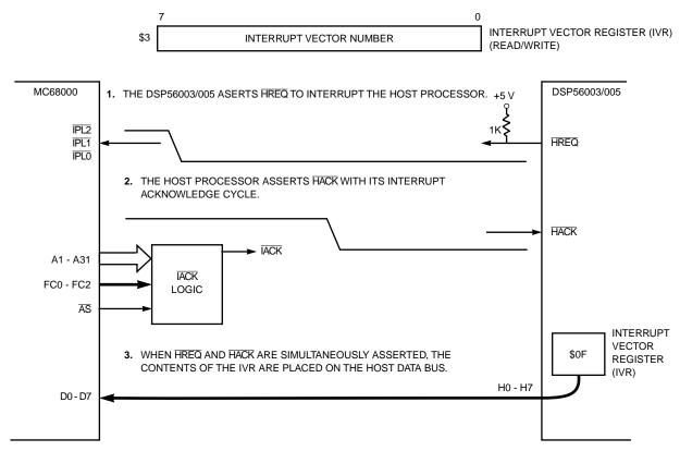
Figure 5-16 Interrupt Vector Register Read Timing
