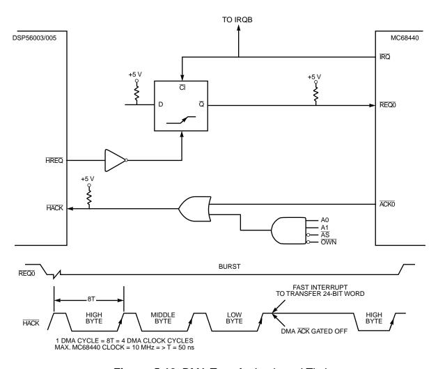
Figure 5-18 DMA Transfer Logic and Timing
