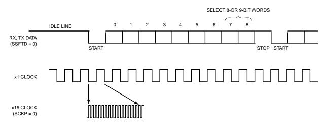
Figure 6-11 16x Serial Clock
