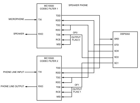
NOTE: SC0 and SC1 are output flag 0 and 1 used to software select either filter 1 or 2.
