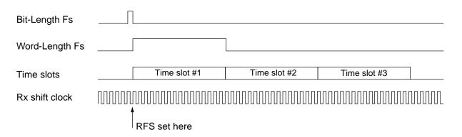
When RFS is clear and a word is received, it indicates (only in network mode) that the frame sync did not occur during reception of that word. RFS is useful in network mode to identify the start of the frame. This feature is illustrated in a typical receive interrupt handler:
