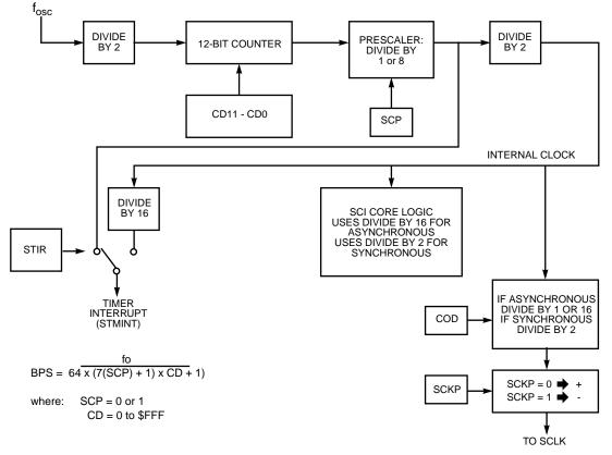
Figure 6-12 SCI Baud Rate Generator
