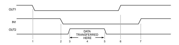
Figure C-7 (4-13) Two DSPs with External Bus Arbitration Timing
