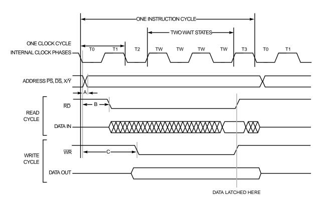
Figure 4-7 External Memory Interface Bus Operation with Two Wait States
