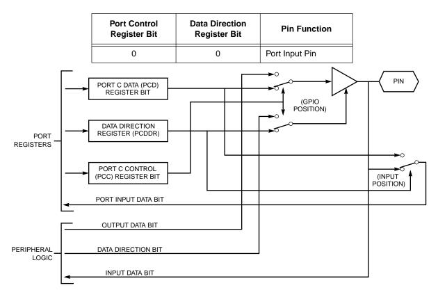
Figure 7-4 Port C I/O Pin Control Logic
