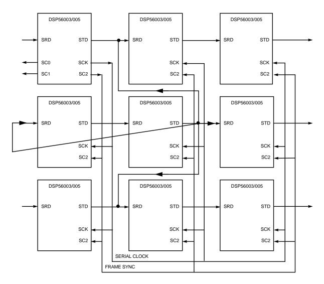
Figure 7-61 SSI Parallel Processing — Nearest Neighbor Array
