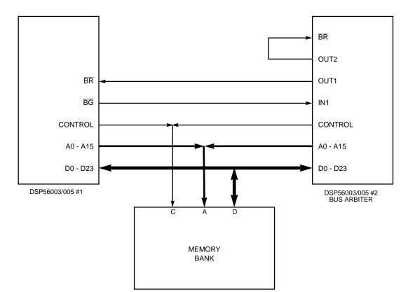
**Figure 4-12** Bus Arbitration Using Only  $\overline{BR}$  and  $\overline{BG}$  with Internal Control — DSP56003 Only
