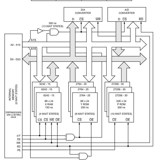
Figure 4-9 Mixed-Speed Expanded System
