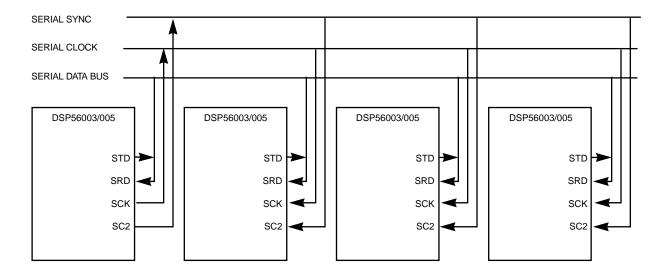
Figure 7-62 SSI TDM Bus DSP Network
