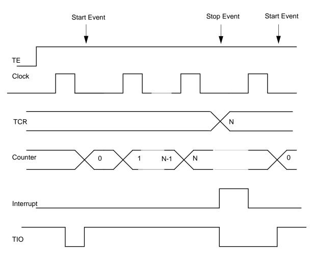
Figure 8-8 Mode 4 — Pulse Width Measurement Mode (INV=0)
