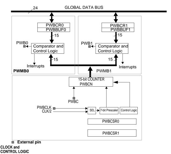
Figure 9-4 PWMB Block Diagram
