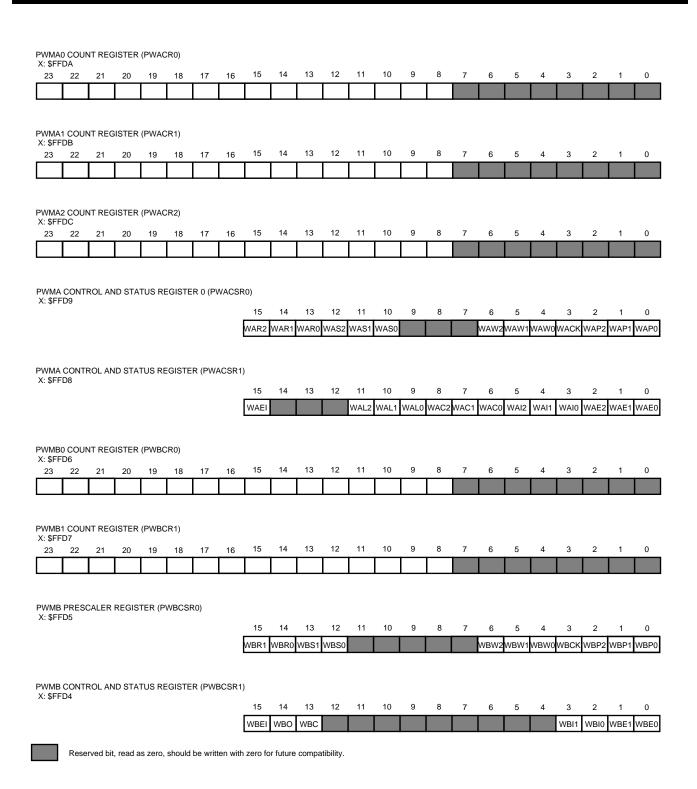
Figure 9-5 PWM Programming Model
