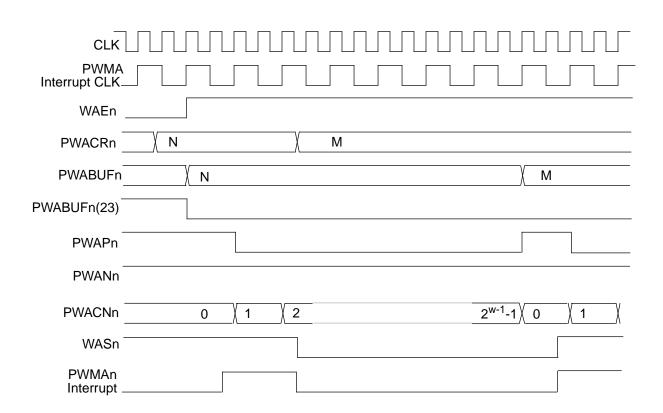
Figure 9-10 PWMA Timing — Internal Clock, Internal Carrier, N=\$7FFF, w=16
