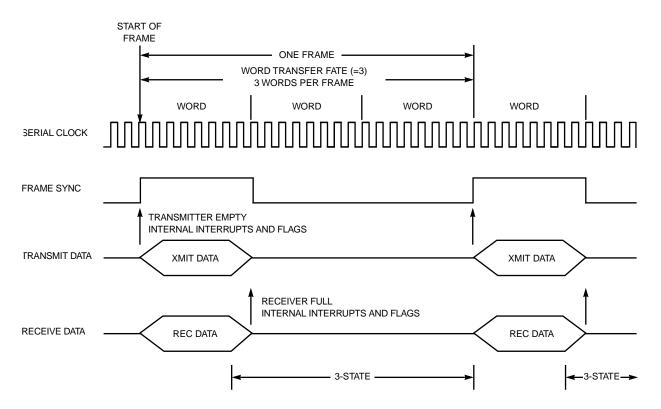
Figure 7-27 Synchronous Communication
