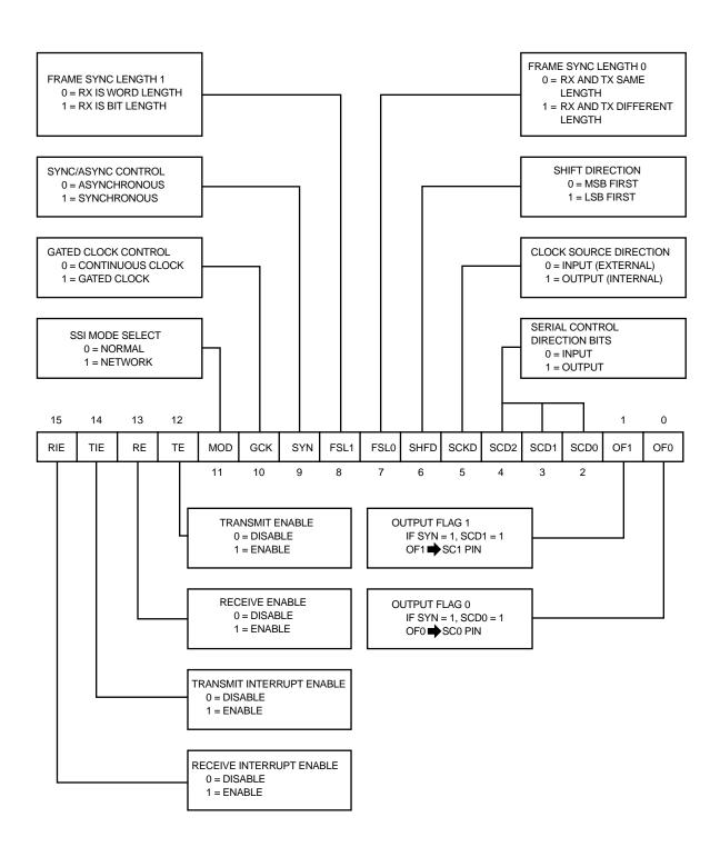
Figure 7-17 SSI CRB Initialization Procedure
