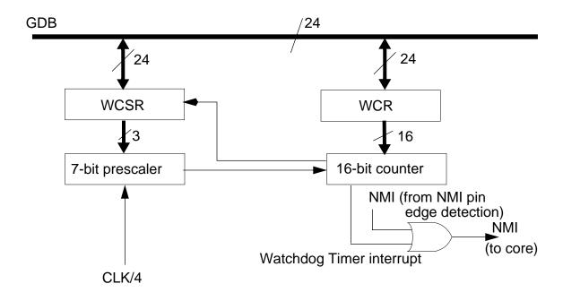
Figure 10-1 16-bit Timer Module Block Diagram
