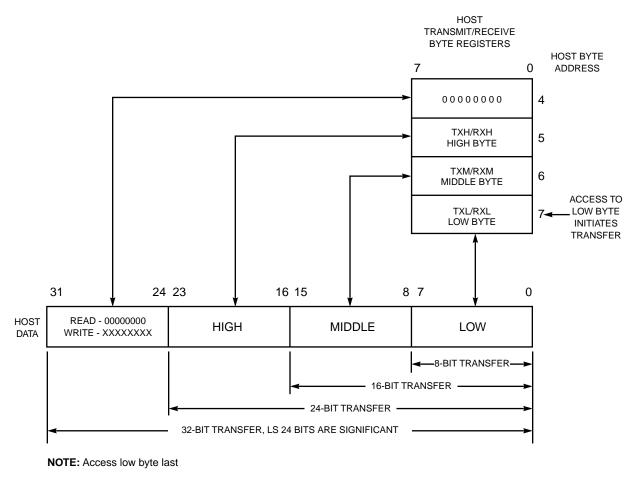
Figure 5-30 Transmit/Receive Byte Registers
