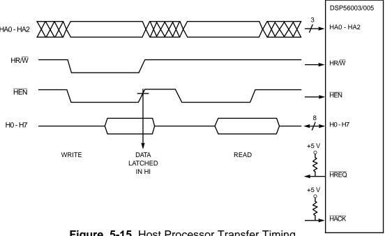
Figure 5-15 Host Processor Transfer Timing
