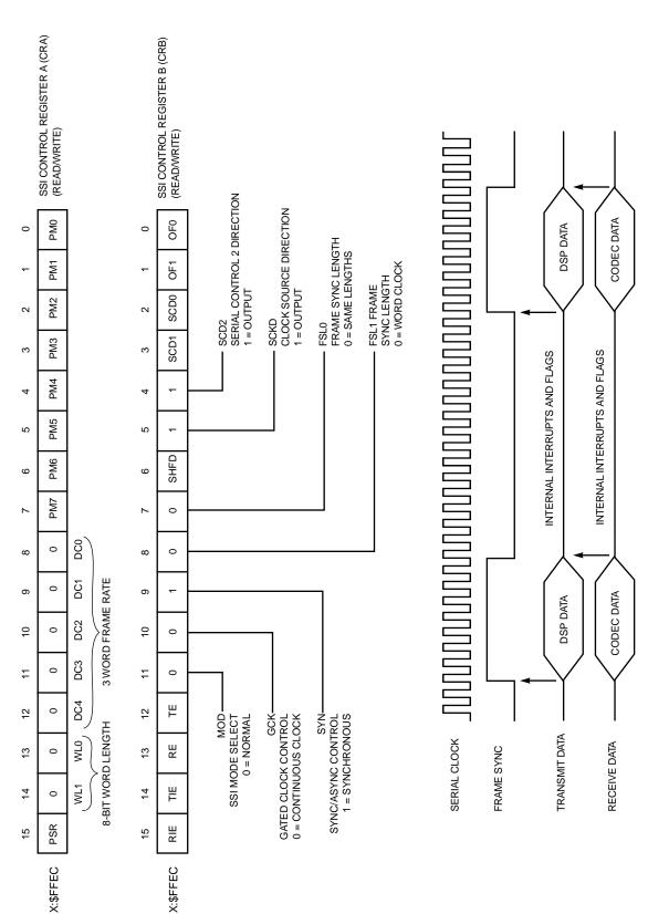
Figure 7-34 Normal Mode Initialization for FLS1=0 and FSL0=0
