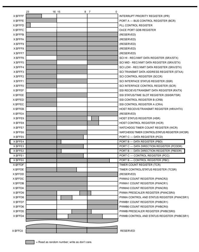
Figure 5-5 On-Chip Peripheral Memory Map
