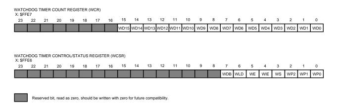
Figure 10-2 Watchdog Timer Module Programming Model
