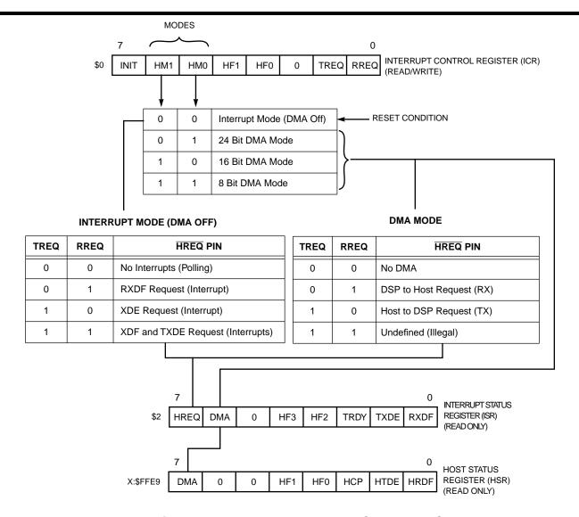
Figure 5-39 Host Bits with TREQ and RREQ
