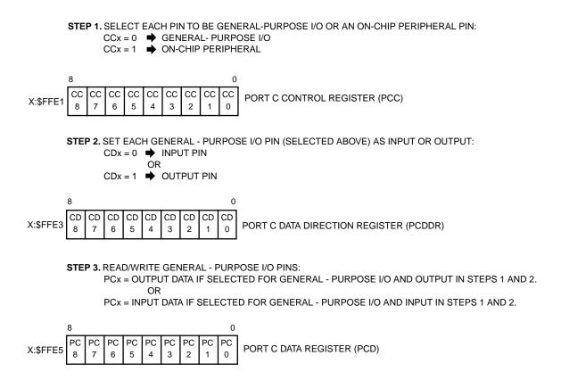
Figure 6-7 I/O Port C Configuration
