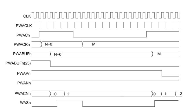
Figure 9-8 PWMA Timing — External Clock, External Carrier, N=0
