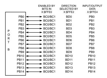
Figure 5-3 Parallel Port B Pinout
