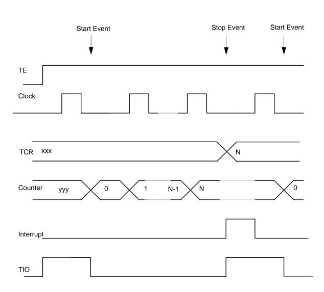
Figure 8-10 Mode 4 — Pulse Width Measurement Mode (INV=1)
