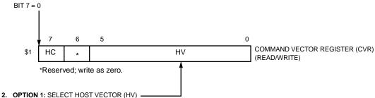
(OPTIONAL SINCE HV CAN BE SET ANY TIME BEFORE THE HOST COMMAND IS EXECUTED. DSP INTERRUPT VECTOR = THE HOST VECTOR MULTIPLIED BY 2. DEFAULT (UPON DSP RESET): HV = \$12 → DSP INTERRUPT VECTOR \$0024
