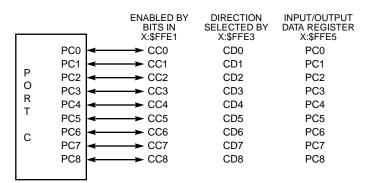
Figure 6-2 Port C GPIO Control
