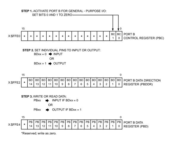
Figure 5-7 I/O Port B Configuration
