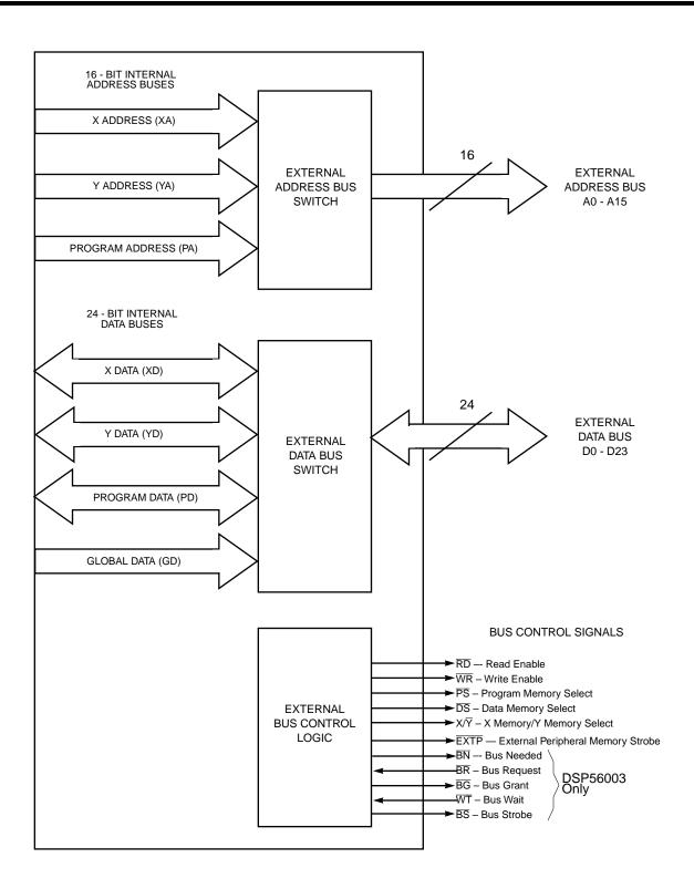
Figure 4-1 External Memory Interface Signals
