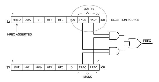
Figure 5-17 HI Interrupt Structure
