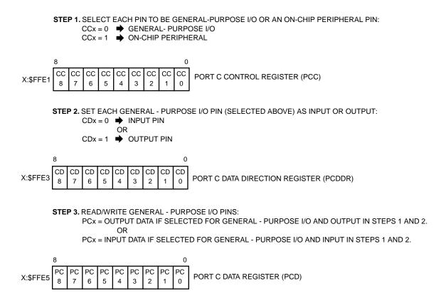
Figure 7-7 I/O Port C Configuration
