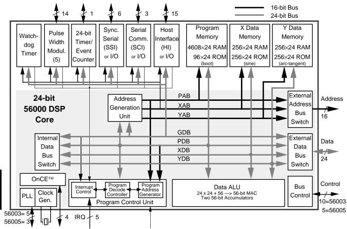
Figure C-1 (1-1) DSP56003/005 Block Diagram
