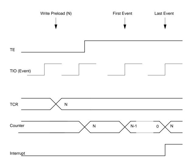
Figure 8-15 Mode 7 — Standard Timer Mode, External Clock (INV=0)
