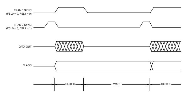
Figure 7-22 Normal Mode, External Frame Sync (8 Bit, 1 Word in Frame)
