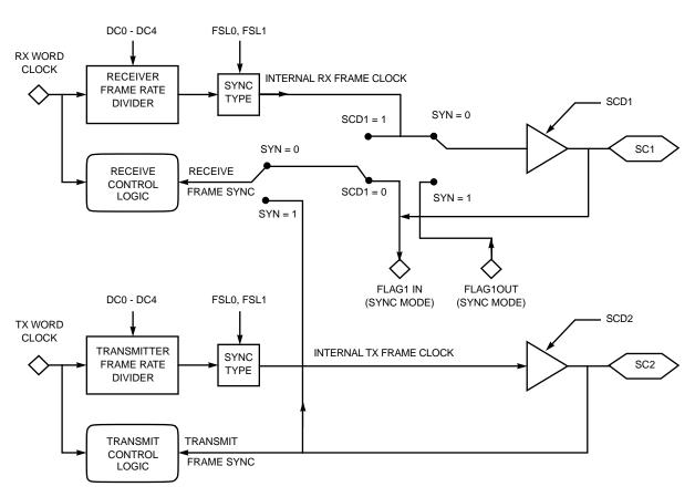
Figure 7-9 SSI Frame Sync Generator Functional Block Diagram
