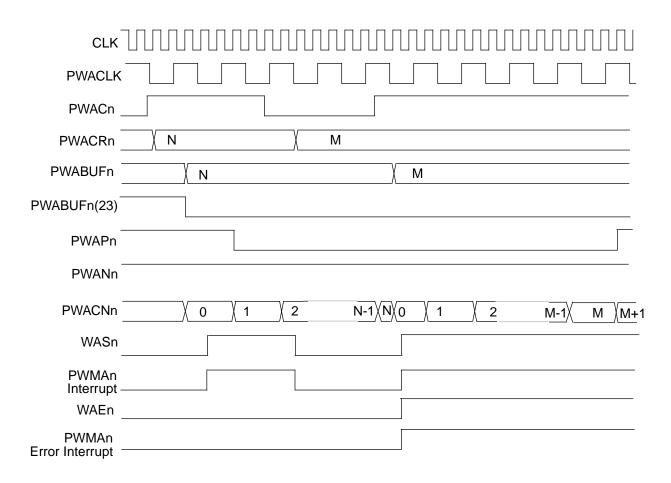
Figure 9-7 PWMA Timing — External Clock, External Carrier, Error
