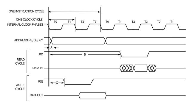
Figure 4-6 External Memory Interface Bus Operation with No Wait States
