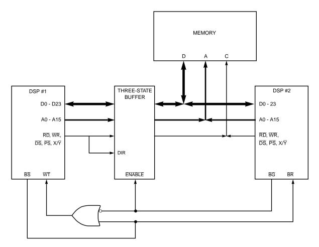
**Figure 4-15** Bus Arbitration Using BR and BG, and WT and BS with No Overhead — DSP56003 Only
