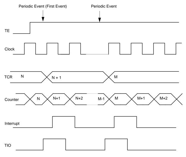
Figure 8-11 Mode 5 — Period Measurement Mode (INV=0)
