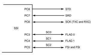
Figure 7-31 Continuous Clock — Synchronous Operation
