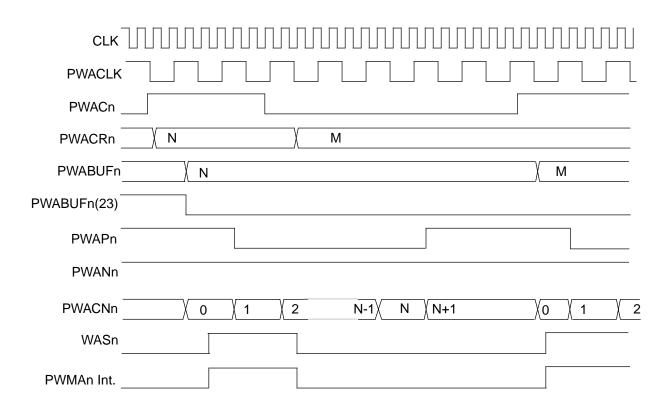
Figure 9-6 PWMA Timing — External Clock, External Carrier, Positive Data
