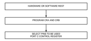
Figure 7-15 SSI Initialization Block Diagram
