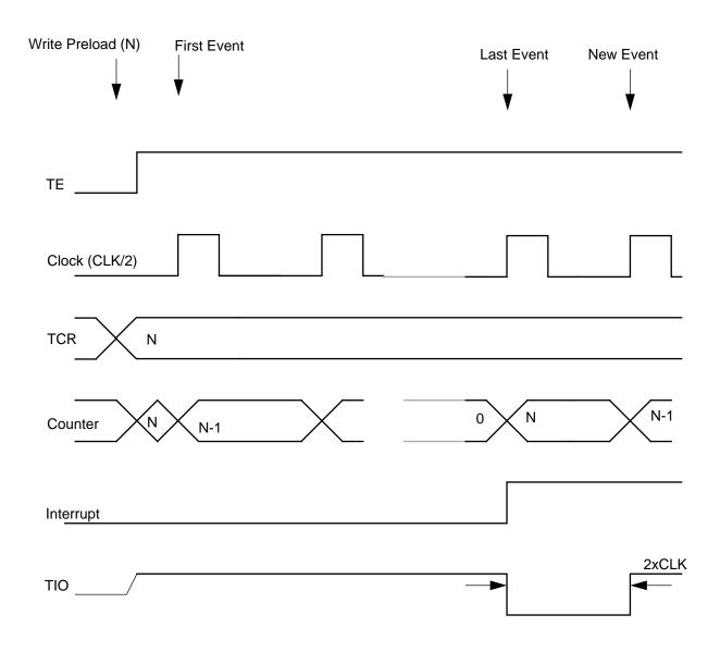
**Figure 8-6** Mode 1 — Standard Timer Mode, Internal Clock, Output Pulse Enabled (INV=1)
