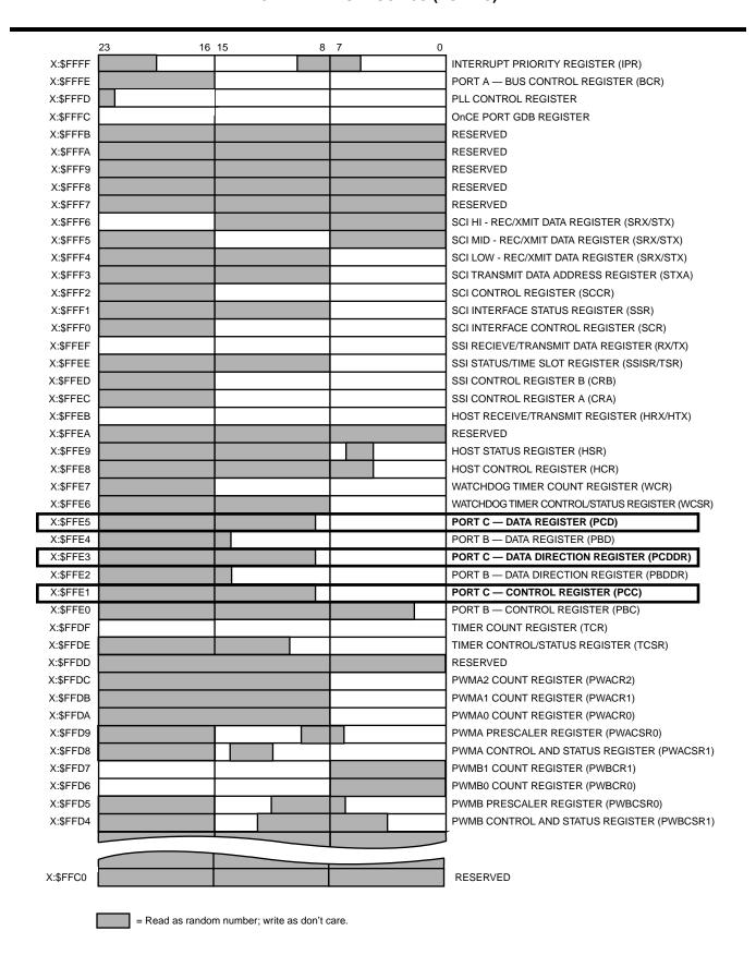
Figure 7-5 On-Chip Peripheral Memory Map
