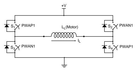
Figure 9-2 DC Motor Control Example Using Pulse Width Modulator A
