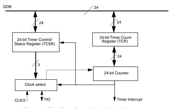
Figure 8-1 Timer/Event Counter Module Block Diagram
