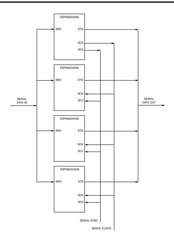
Figure 7-58 SSI TDM Parallel DSP Network
