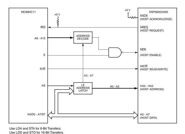
Figure 5-41 MC68HC11 to DSP56003/005 Host Interface
