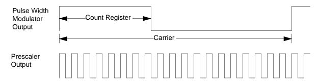
Figure 9-1 Pulse Width Modulator Waveform Controls
