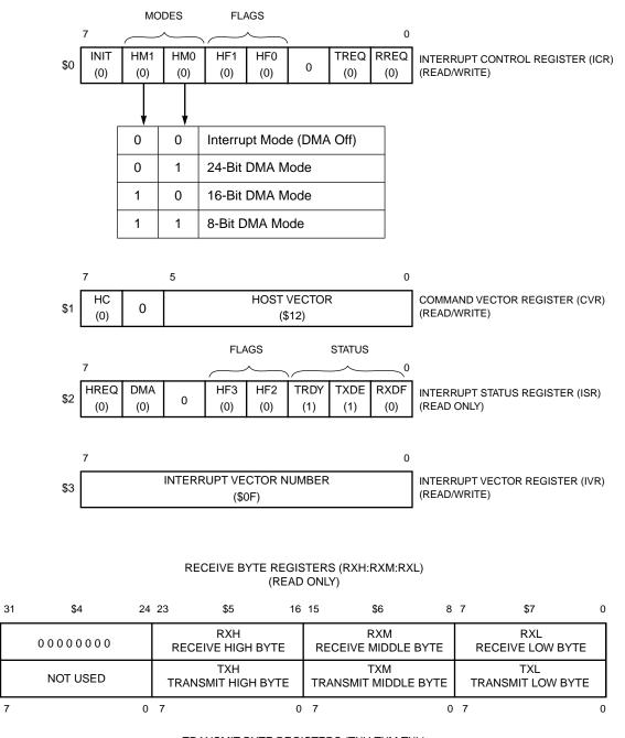
TRANSMIT BYTE REGISTERS (TXH:TXM:TXL) (WRITE ONLY)
