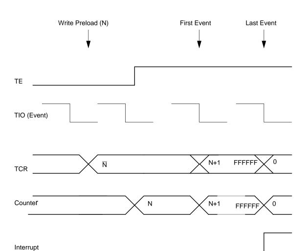
Figure 8-14 Mode 6 — Standard Timer Mode, External Clock (INV=1)
