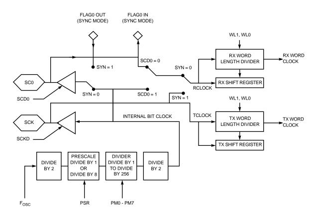
Figure 7-8 SSI Clock Generator Functional Block Diagram
