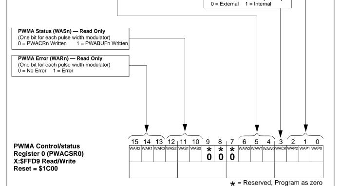
Figure B-39 PWMA Control/status Register 0 (PWACSR0)
