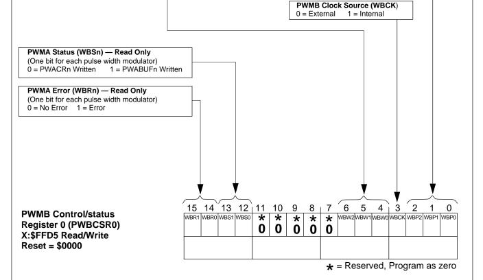
Figure B-43 PWMB Control/status Register 0 (PWBCSR0)
