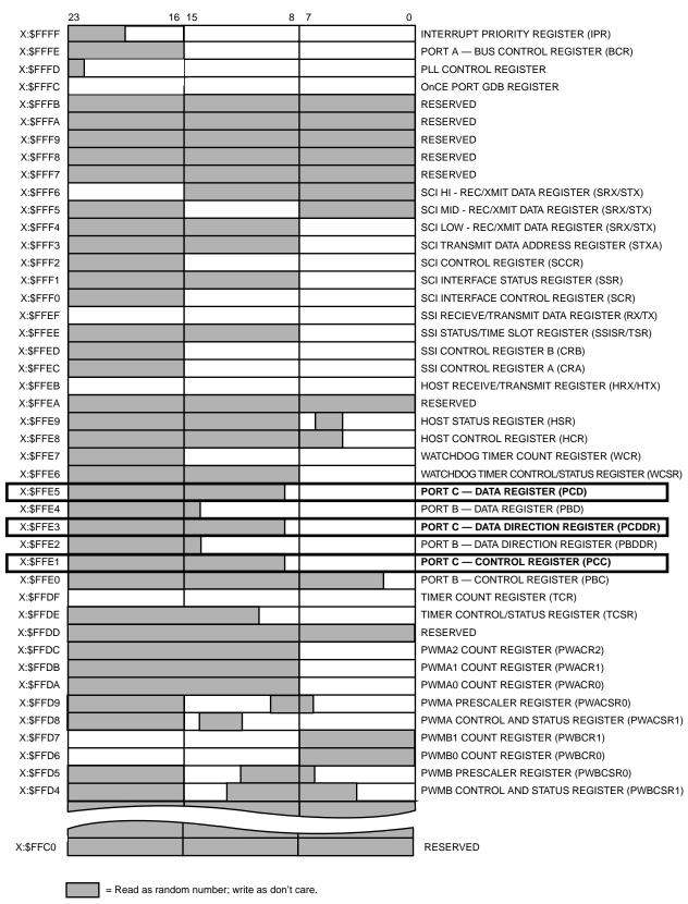
Figure 6-5 On-Chip Peripheral Memory Map
