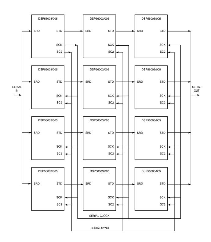
Figure 7-60 SSI TDM Serial/Parallel Processing Array
