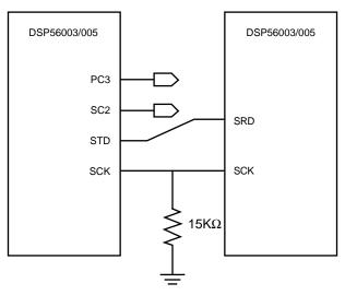
Figure 7-50 On-Demand Mode Example — Hardware Configuration
