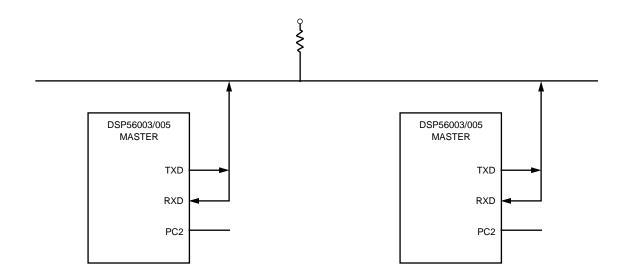
Figure 6-40 Multimaster System Example
