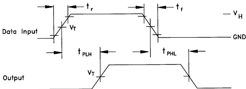
Input and output threshold voltage:
