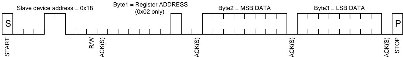
\* Sequential Write is available only for DATA\_M registers(Address 0x02)
