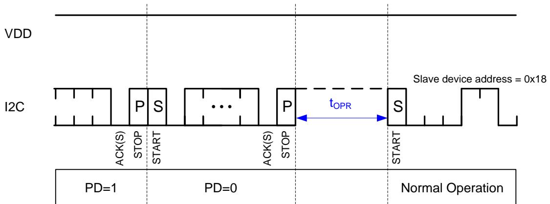
※ DW9718S requires waiting time(delay time) of  $t_{OPR}$  after PD reset takes place.
