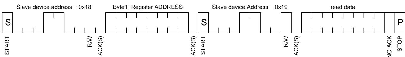
\* In I2C format, Master(ISP, AP etc.) must check the ACK bit before sending the next data.
