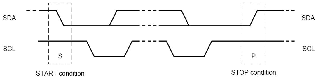
Within the procedure of the I2C-bus, unique situations arise which are defined as START(S) and STOP(P) conditions. A HIGH to LOW transition on the SDA line while SCL is HIGH is one of such unique cases. This situation indicates a START condition. A LOW to HIGH transition on the SDA line while SCL is HIGH defines a STOP condition.
