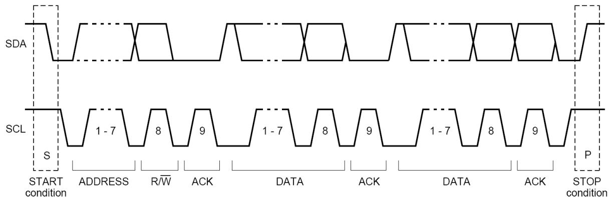
Data transfers follow the above format. After the START condition(S), a slave address is sent. A data transfer is always terminated by a STOP condition(P) generated by the master. However, if the master still needs to communicate on the bus, it can generate a repeated data transfer.
