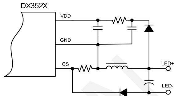
Figure1: Floating ground supply
