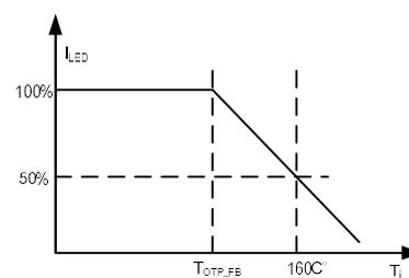
Figure 5: Thermal Foldback Curve
