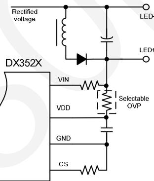
Figure2: low-side switching supply
