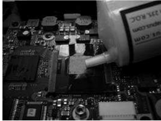
Figure 4-23 Applying silicon grease
