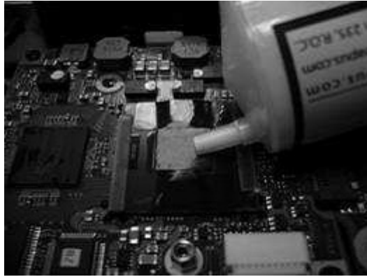
Figure 4-21 Applying silicon grease
