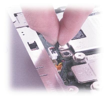
NOTICE: Carefully separate the palm rest from the base plastics to avoid damage to the palm rest.
