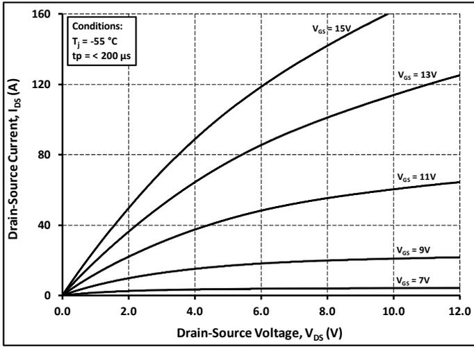
Figure 1. Output Characteristics  $T_j = -55\text{ }^\circ\text{C}$
