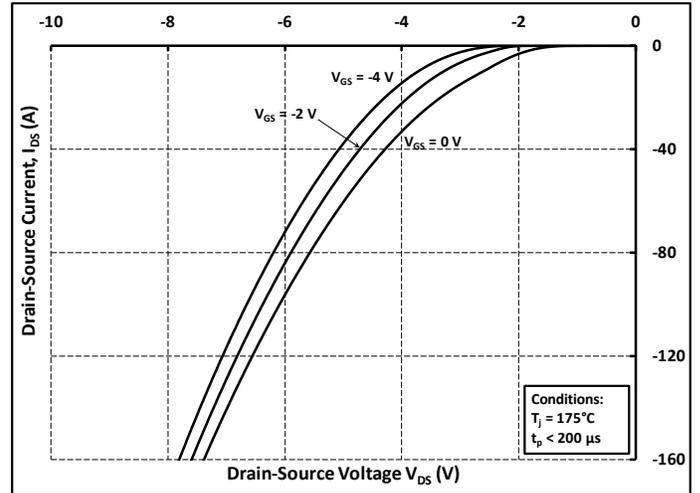
Figure 10. Body Diode Characteristic at 175 °C
