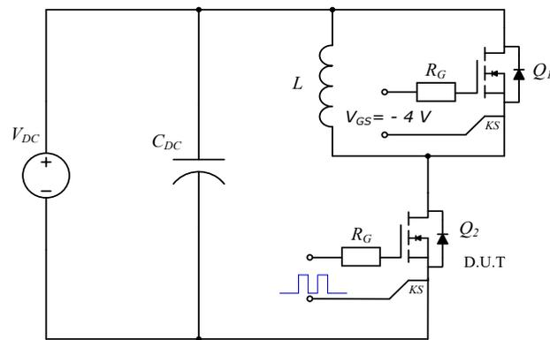
Figure 29. Clamped Inductive Switching Waveform Test Circuit
