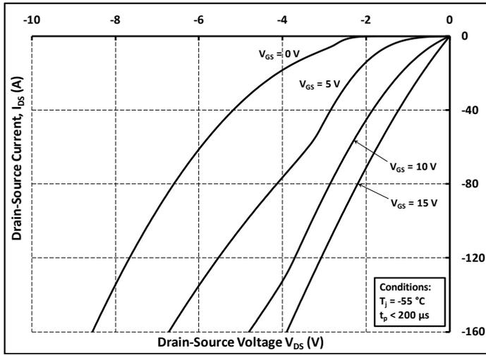
Figure 13. 3rd Quadrant Characteristic at -55 °C
