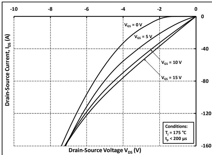
Figure 15. 3rd Quadrant Characteristic at 175 °C
