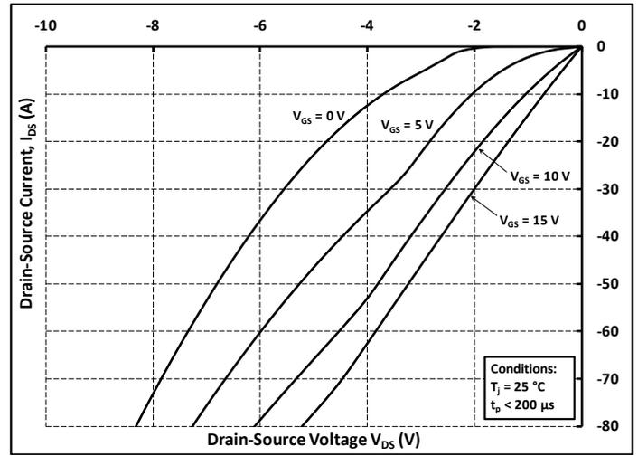
Figure 14. 3rd Quadrant Characteristic at 25 °C
