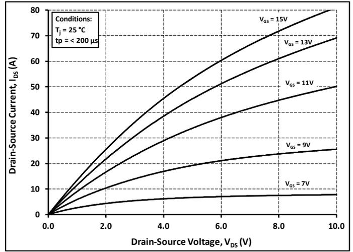
Figure 2. Output Characteristics  $T_j = 25\text{ }^\circ\text{C}$
