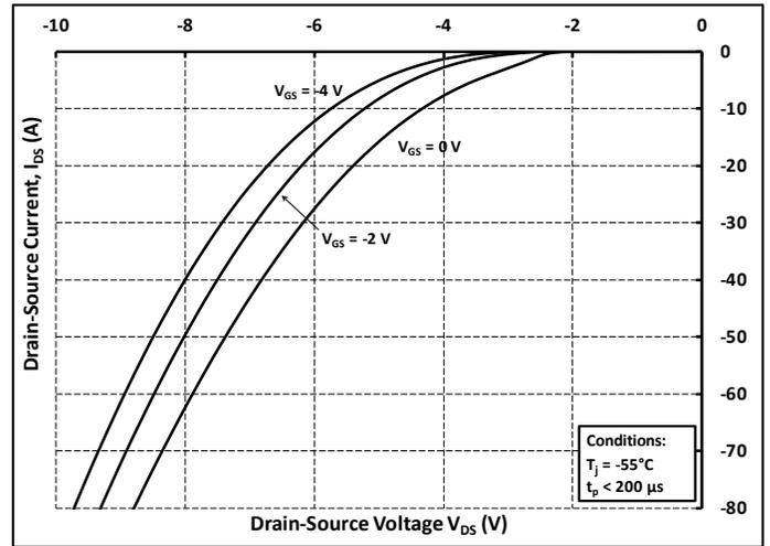
Figure 8. Body Diode Characteristic at -55 °C
