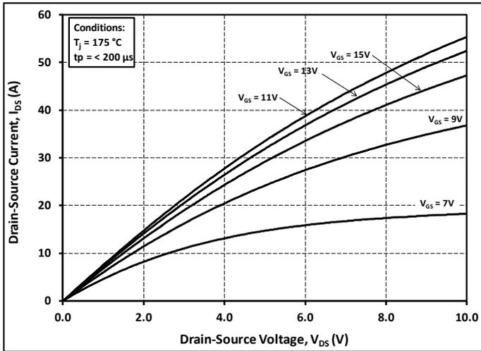
Figure 3. Output Characteristics  $T_j = 175\text{ }^\circ\text{C}$
