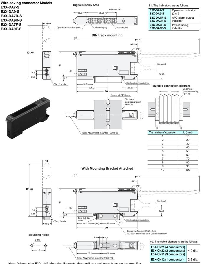
**Note:** When using E39-L143 Mounting Brackets, there will be small gaps between the Amplifier Units if they are mounted side by side.
