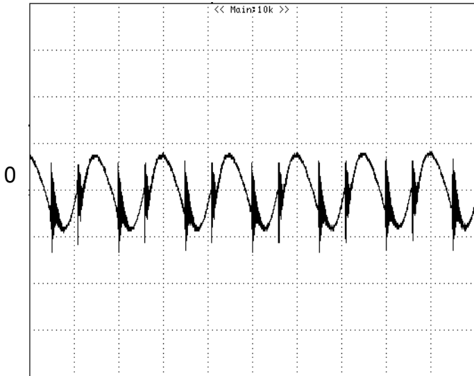
Figure 14: Output voltage ripple at nominal input voltage and rated load current ( I_o=25A ) (10 mV/div, 2 us/div) Load capacitance: 1 \mu F ceramic capacitor and 10 \mu F tantalum capacitor. Bandwidth: 20 MHz. Scope measurements should be made using a BNC cable (length shorter than 20 inches). Position the load between 51 mm to 76 mm (2 inches to 3 inches) from the module
