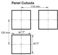
Note: 1. Recommended panel thickness is 1 to 8 mm.
