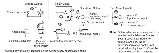
The input power supply depends on the power supply specification of the Controller and is either 100 to 240 VAC or 24 VAC/DC (no polarity). Order the P2CF-11 or P3GA-11 Socket separately. (See page 14.)
