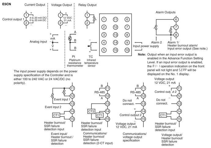
Terminals 11 to 15 do not exist on models without an Option Unit (heater burnout detection, control output 2, event inputs, or communications). Terminal applications depend on the model of the Option Unit.
