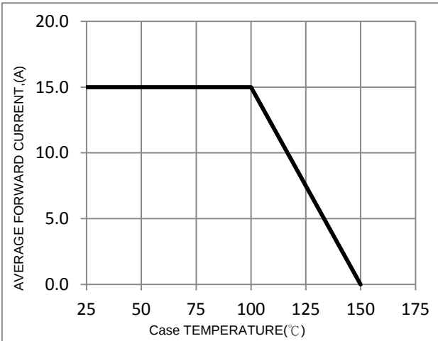
FIG. 1-Typical Forward Current Derating Curve
