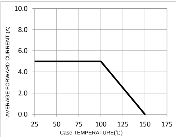
FIG. 1-Typical Forward Current Derating Curve
