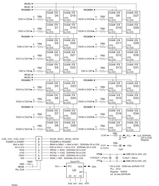
1. The SDA pull-up resistor is required due to the open-drain/open-collector output.
