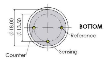
All dimensions are in millimeters. All tolerances are ±0.2mm.
